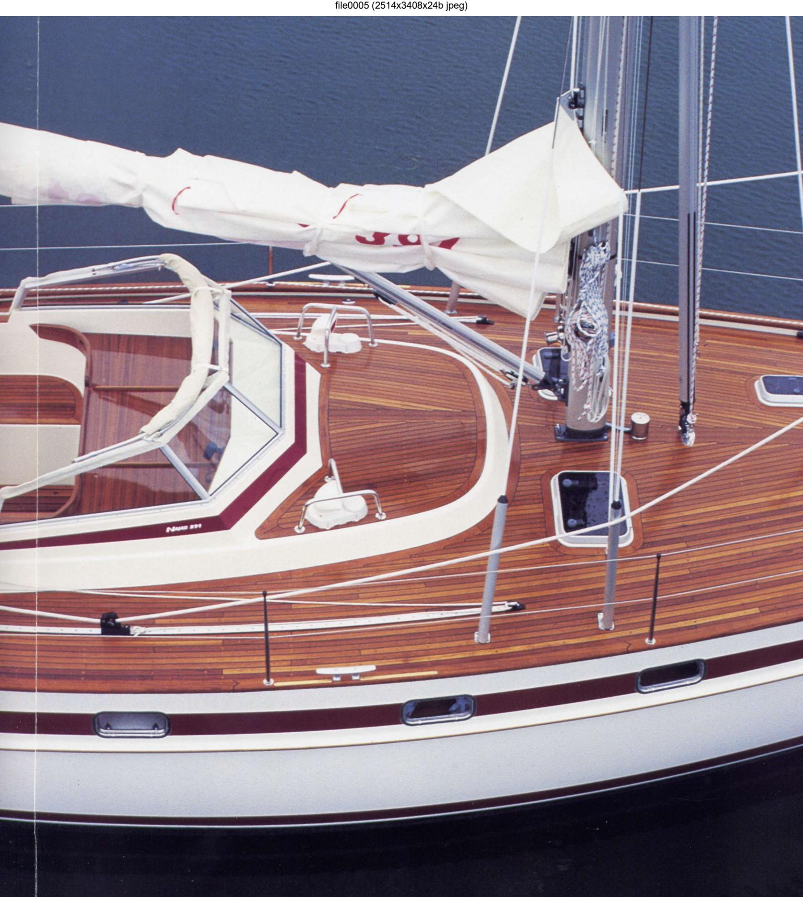
The Najad 391 is designed with a large, uncluttered, flush teak deck. The teak planks are curved to follow the sheer of the hull with solid teak fitted around the outer deck edge and hatches.
